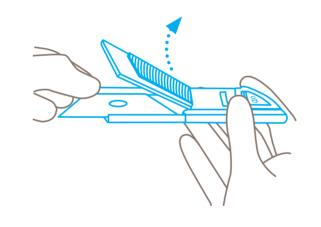
Hold the **blunt** side of the blade and use it to lift the blade cover upwards. The cover remains in the open position.
