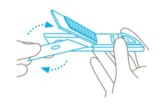
Reverse or replace the blade. Make sure you place the blade **exactly** on the locating lobe.
